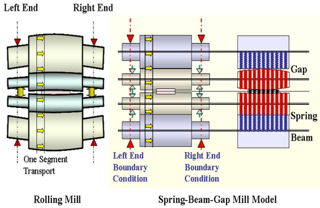
Figure 1: Spring-Beam-Gap Mill Model
